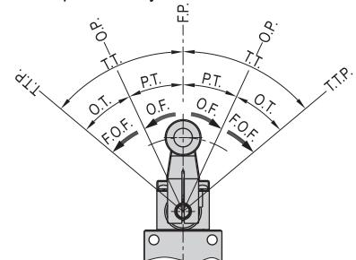
F.P. Free position: the position of control head when no external force applied;
