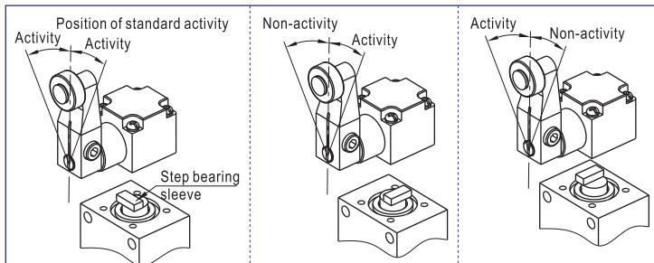
2. The rolling wheel could be installed at the inside of leverage
