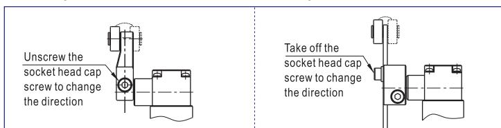
3. Installation position of leverage could be changed
